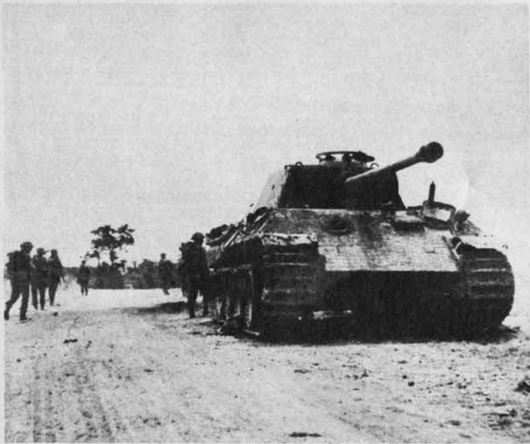
Panther design was influenced by that of Russian T-34. Bow is long and sloping. Forward set of turret makes tank seem to lunge ahead.
